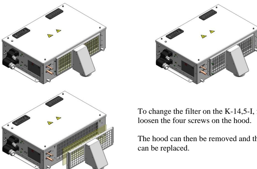
To change the filter on the K-14,5-I, first loosen the four screws on the hood.
