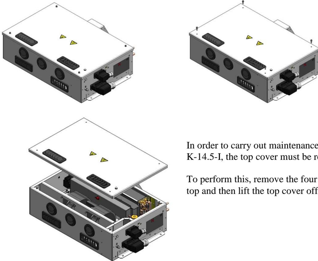
In order to carry out maintenance work on the K-14.5-I, the top cover must be removed first.
